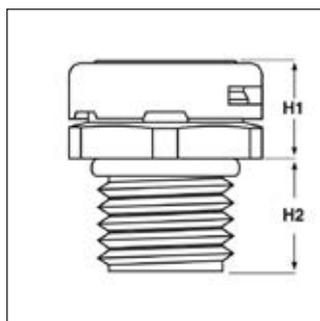
**Materiale:** tappi in poliammide 6, membrana in PES (Polietersulfone), O-Ring in NBR.
