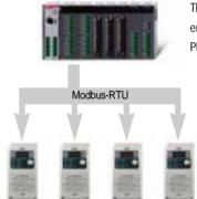
The optional modbus communication enables controlling drives through PLC and other controlling devices.
