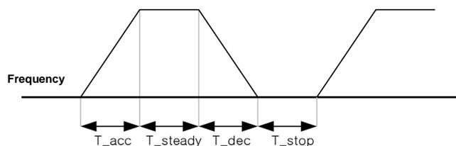
Figure 8-9 Example 1 of setting braking resistor usage
