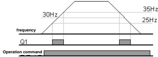
Figure 7-34 FDT-3 when the detected frequency width is 10 Hz and the detected frequency is 30 Hz
