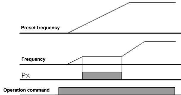
Figure 6-10 Frequency HOLD of analog command
