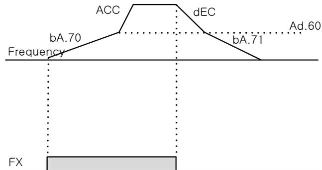
Figure 6-19 Changing multi-step Acc/Dec time by setting Acc/Dec time transition frequency
