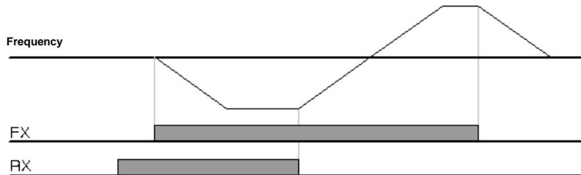
Figure 6-13 Terminal Block Operating Command 2
