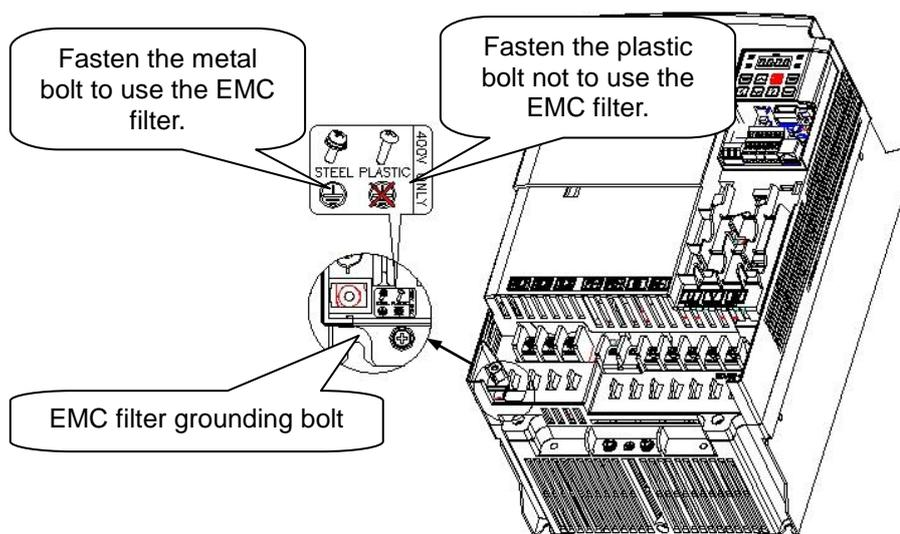
Figure 4-8 Disabling 5.5-22 kW or less EMC filter function
