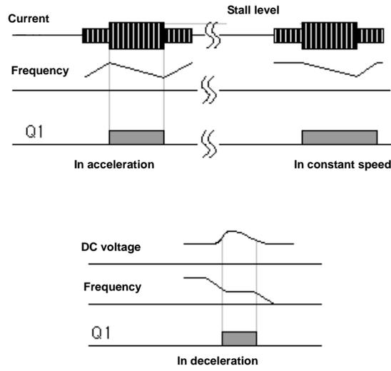
Figure 8-4 Stall protection during acceleration, deceleration and at a constant speed
