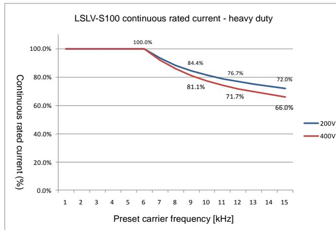
Figure 2-5 Continuous rated current for heavy load
