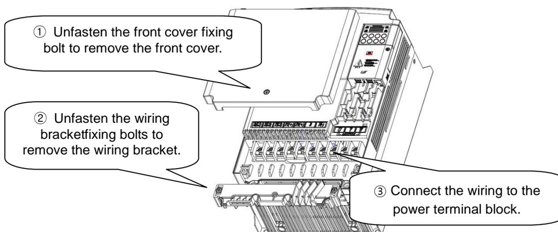
Figure 4-2 Removing the front cover and wiring bracket (15 kW 200 V - 22 kW 200/400 V)
