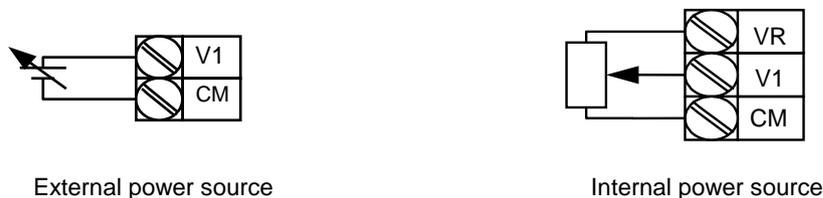
Figure 6-1 Frequency setting by voltage input into the terminal block
