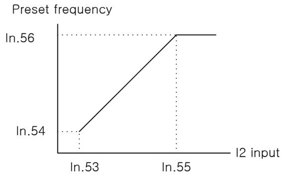
Figure 6-8 Setting the gradient of output frequency and offset value for the magnitude of current
