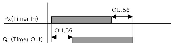
Figure 7-27 Timer function of multi-function input terminal
