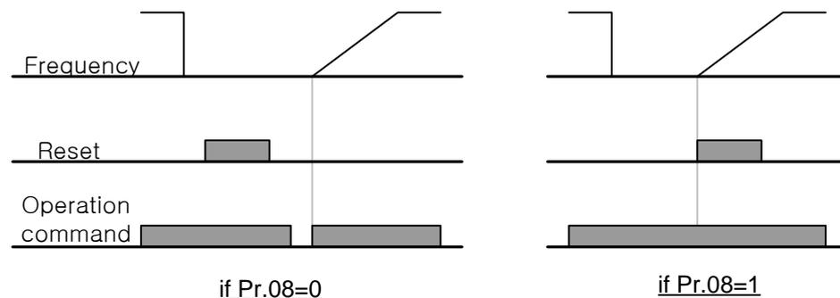
Figure 6-15 Comparison of the RST Restart function when it is set to Pr.08 = 0 or Pr.08 = 1
