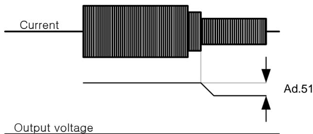
Figure 7-20 Manual energy saving operation
