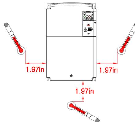
Figure 3-1 Positions for measuring ambient temperature
