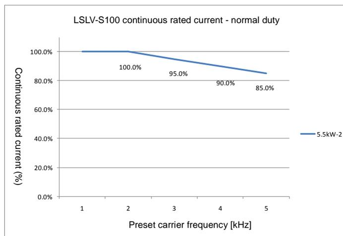
Figure 2-6 Continuous rated current for light load (5.5 kW 200 V)
