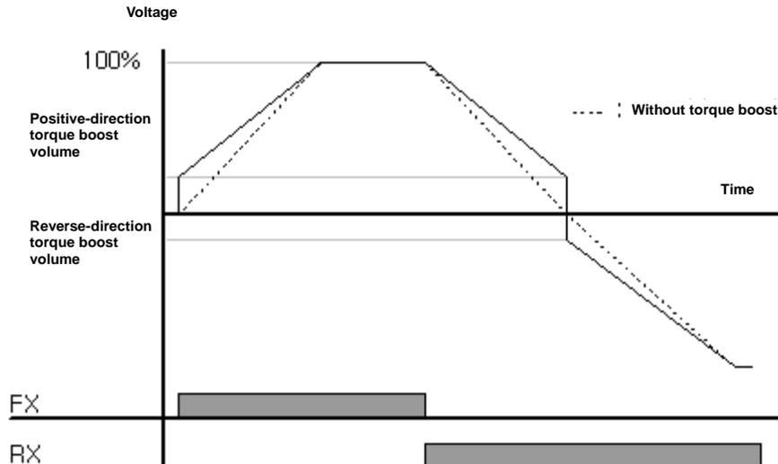
Figure 6-26 Manual torque boost
