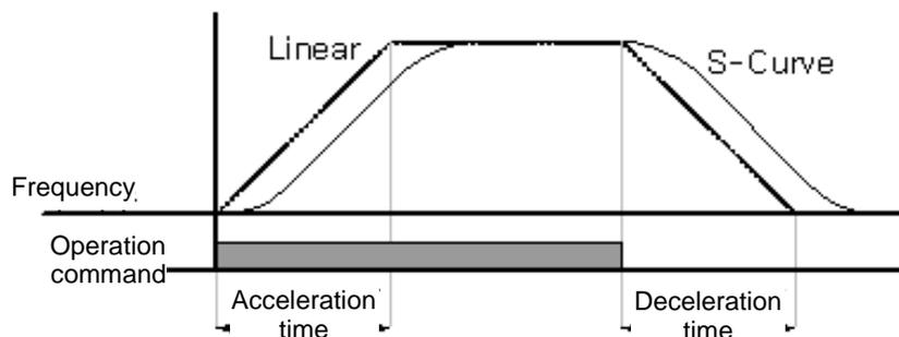
Figure 6-20 Setting Acc/Dec pattern
