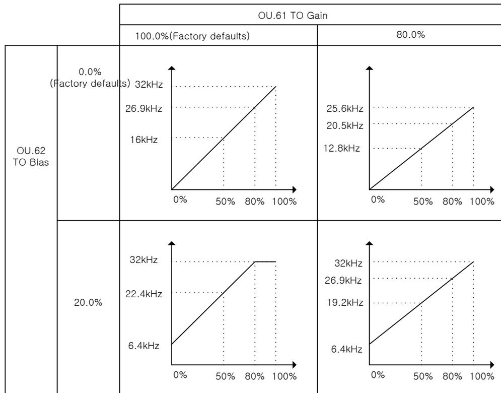
Figure 7-31 Pulse output change when dr.20 Max Freq is 60 Hz and the current output frequency is 30 Hz
