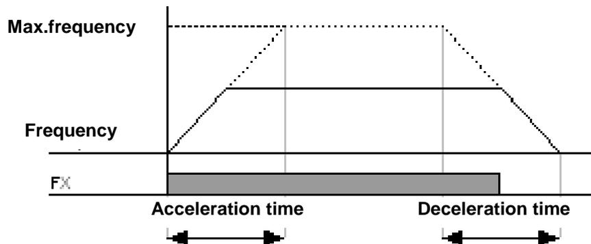
Figure 6-16 Setting Acc/Dec time
