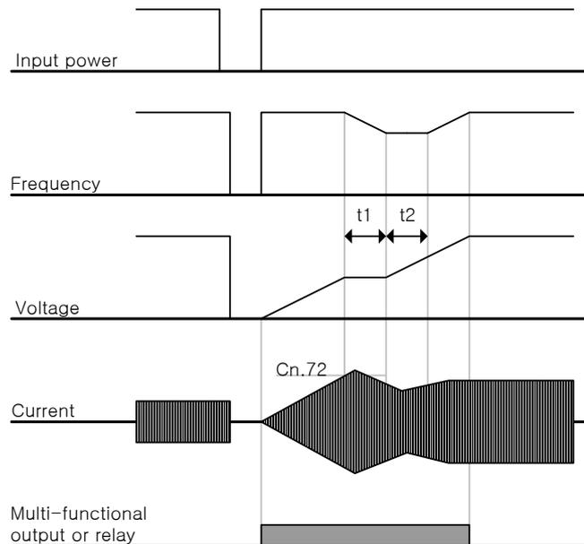
**Figure 7-21 Speed search operation after instantaneous power interruption occurs and power returns**
