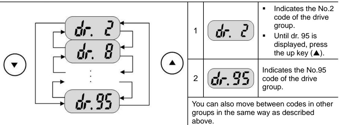
When using the up key (▲) or down key (▼) to move between codes in each group, sometimes the code number skips instead of increasing or decreasing by 1. This is because the inverter program keeps the number empty, reserving them for functions to be added later, or it has hidden the functions not used by the users. For detailed information, refer to Chapter 10 Function Display List.
