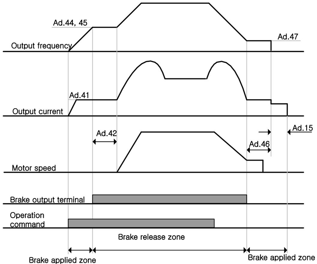
Figure 7-28 Brake operation sequence
