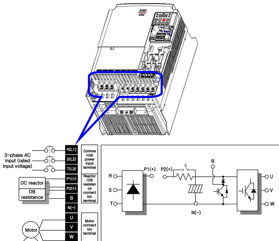
Note: Necessary screen around motor wires not shown for clarity
