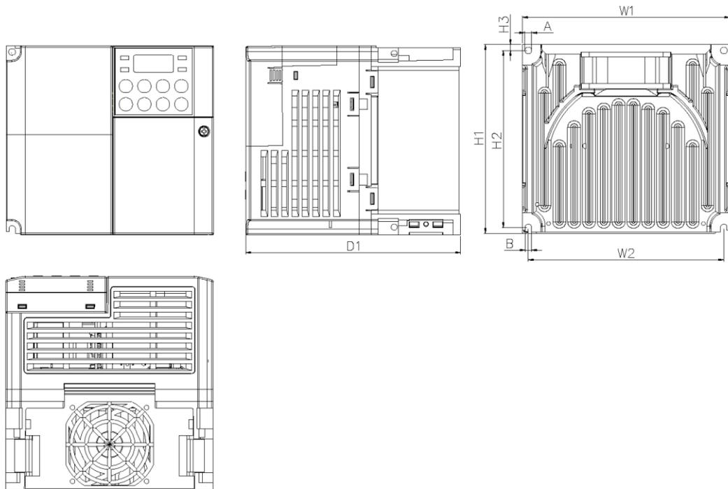
Figure 2-3 LSLV0022 S100 (single-phase 200 V), LSLV0037 S100 – 0040 S100 (3-phase 200 V/3-phase 400 V)
