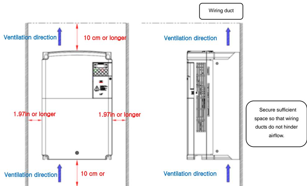
Figure 3-2 Ambient spacing
