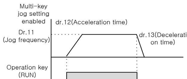
Figure 7-5 Keypad based jog operation
