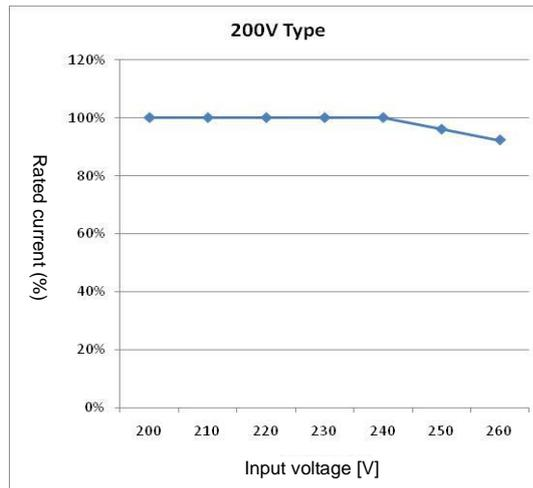
Figure 2-7 3-phase 200 V type continuous rated current
