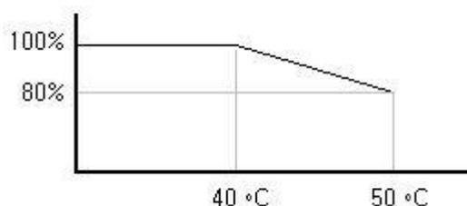
**Figure 7-23 Rated current limits for ambient temperature if the inverter operates at normal duty**
