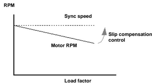
Figure 7-14 Slip compensation operation
