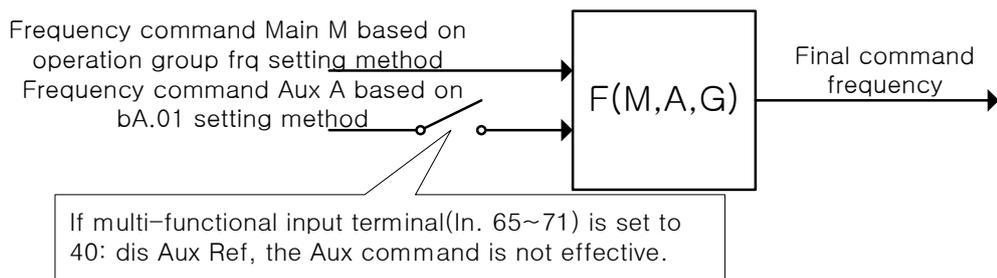
**Figure 7-1 Setting the override frequency using the aux frequency command**
