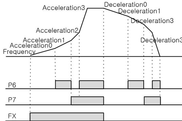
Figure 6-18 Setting multi-step Acc/Dec time using multi-function terminals
