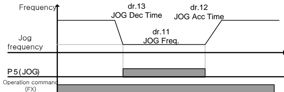
Figure 7-3 Terminal block based jog operation
