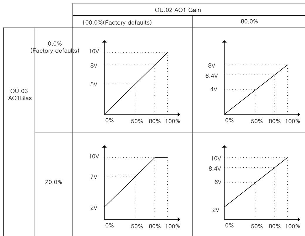
Figure 7-30 Analog voltage output change when dr.20 Max Freq is 60 Hz and the current output frequency is 30 Hz
