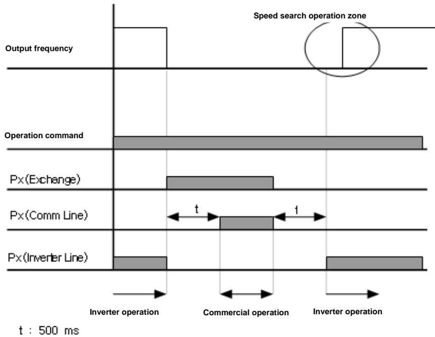
Figure 7-25 Relay operation sequence
