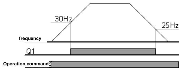
Figure 7-35 FDT-4 when the detected frequency width is 10 Hz and the detected frequency is 30 Hz
