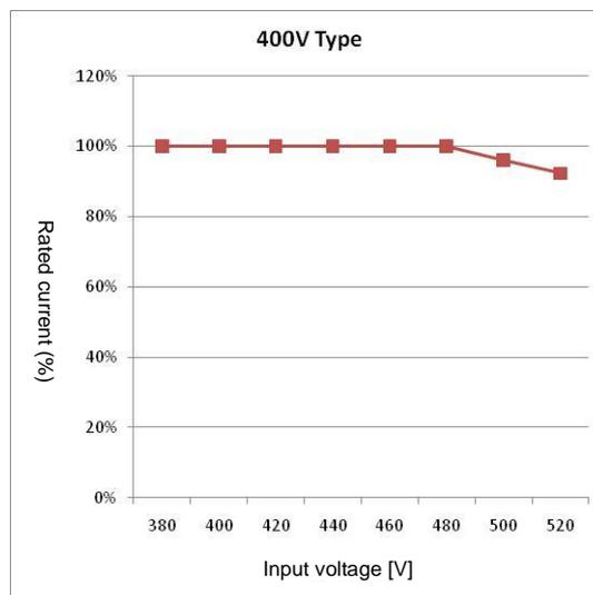
Figure 2-8 3-phase 400 V type continuous rated current
