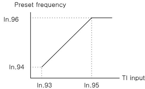
**Figure 6-9 Setting the gradient of output frequency and offset value for the magnitude of pulse**
