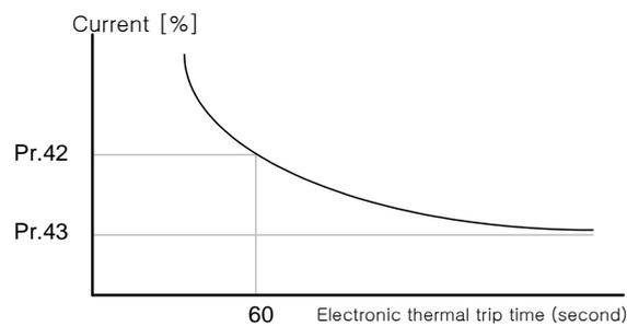
**Figure 8-2 Electronic thermal protection function**
