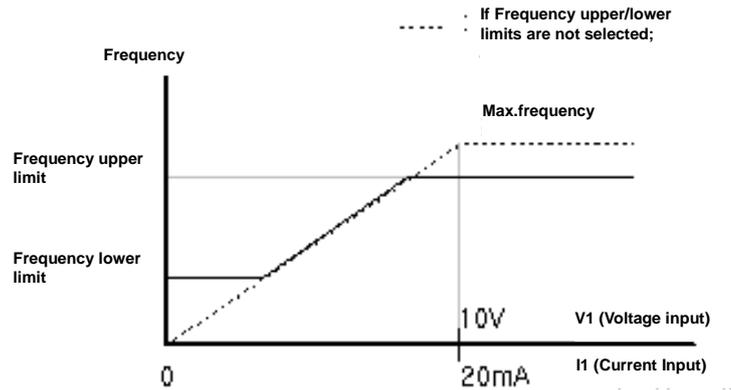
Figure 6-32 Limiting frequency using the upper and lower limit of frequency
