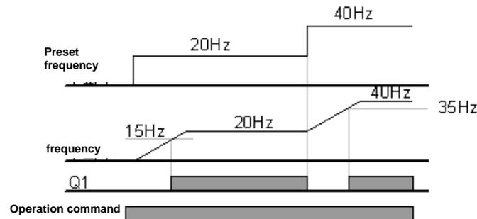
Figure 7-32 FDT-1 when the detected frequency width is set to 10 Hz
