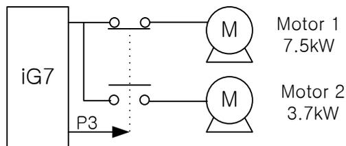
**Figure 7-24 Usage example: 2nd motor operation function**
