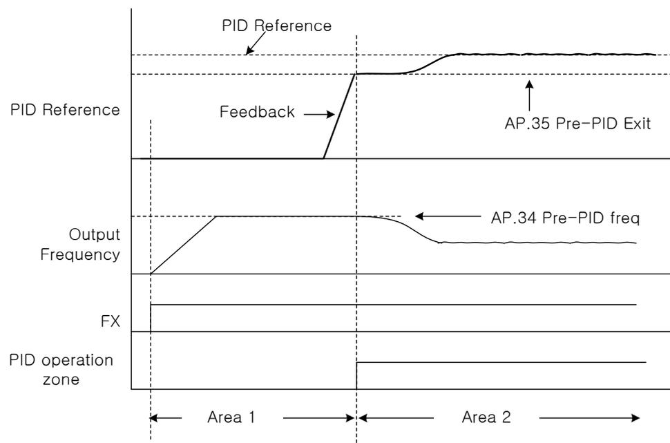
Figure 7-16 Pre-PID operation
