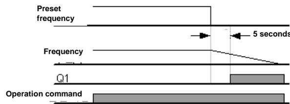
**Figure 8-8 Set Pr.15 AI Lost Level to 1, Pr.12 Lost Cmd Mode to 2, Pr.13 Lost Cmd Time to 5 sec**
