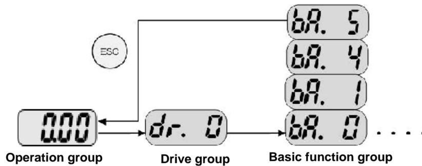
For the ESC key, the initial value (dr.90) is preset to 0 (move to the initial position). Therefore, if you press the ESC key in any code position in a group, you will be moved to the first position of the operation group. For other functions of the ESC key, refer to 5.11 Using the Multi-keys.
