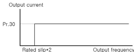
Figure 8-12 Setting Heavy load rate (heavy duty)
