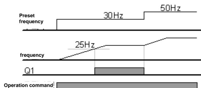
Figure 7-33 FDT-2 when the detected frequency width is 10 Hz and the detected frequency is 30 Hz
