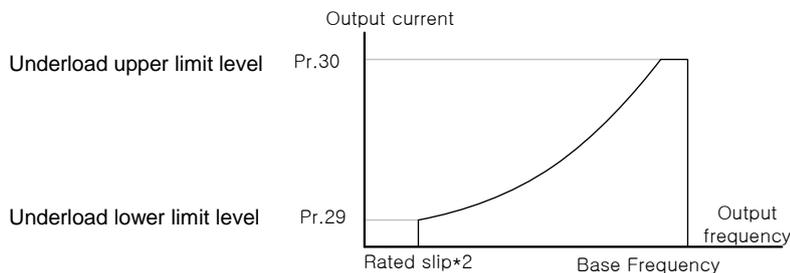
Figure 8-11 Setting underload rate (normal duty)
