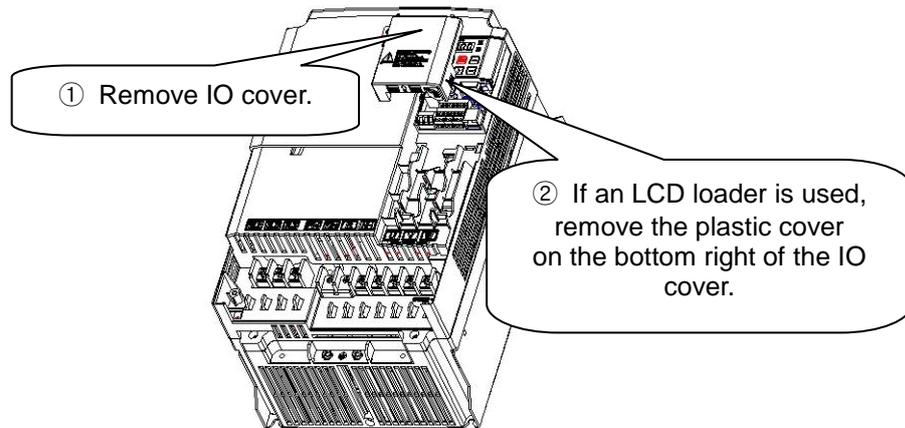
Figure 4-3 Removing IO bracket
