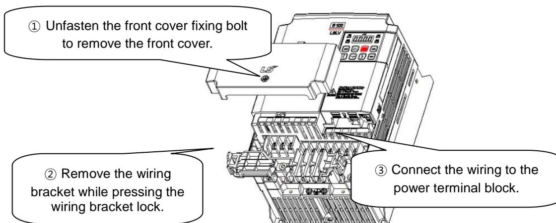
Figure 4-1 Removing the front cover and wiring bracket (5.5 kW 200/400 V - 15 kW 400 V)
