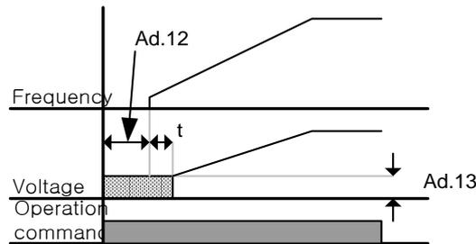
Figure 6-28 Start after DC braking
