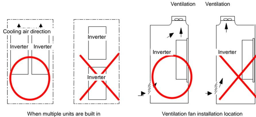
**Figure 3-3 Ventilation fan and inverter installation locations**
