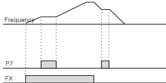
Figure 6-22 Acc/Dec stop command using the terminal P7
