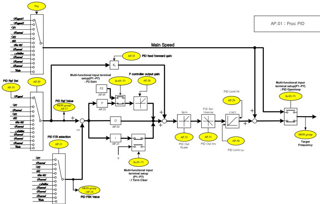
Figure 7-15 PID control block diagram
